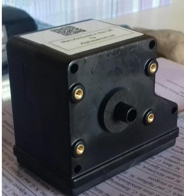
Figure 1. OPC-N3 particulate is used to measure particles.
